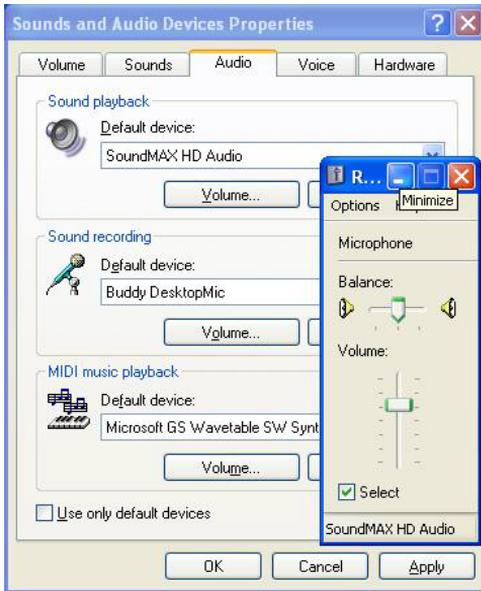
Adjust the slider for the microphone control 2/3 the way towards the top peak.
