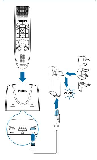
→ During charging, the battery LED on the SpeechMike and on the docking station glow orange.
